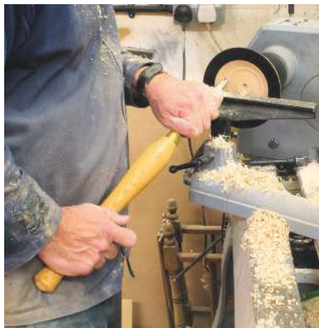
▲ Pic.12 A common mistake is to keep the gouge horizontal when hollowing a bowl. To keep the bevel in contact with the inside curve, the tool handle will need to drop throughout the shaping process
